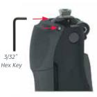
Installing the Knee Cap b. Install Knee Cap as indicated below. Tighten the 2 socket head cap screws using the 3/32"Hex Key.
