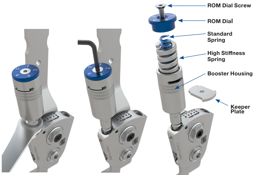
Figure 4. Adjust the booster to 15° ROM.
