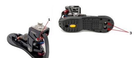
Remove screws labeled 1 (3mm hex) and 3 (5mm hex). Swap sole plates and assemble using Blue Loctite and torque bottom screws to 95 inch lbs. (the heel guard stays attached to sole plate)
