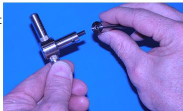
**FIGURE 8A:** Insert hex shaft driver into shaft.
