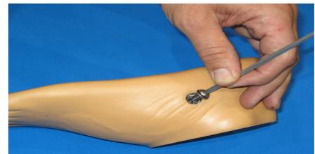
FIGURE 14: Installing the screw and washer.
