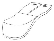
**5.** Glue Soleflex (moderately dense) crepe around the outside of the heel plate and sand the top and bottom to match the contour of heel plate and the wedge created in step 4.
