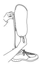
**4.** Bond the socket to the pylon using Fabtech PLUSeries® Composite Adhesive as shown. Check the alignment and correct by rebonding the setup before proceeding to the next step.
