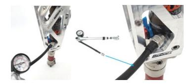
**Note:** when threading air pump onto filler valve, the pressure from inside the shock pressurizes pump which reduces the air pressure by around 5-8psi. Gauge is accurate when removing from valve.
